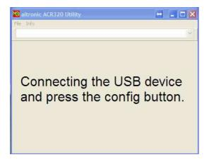
To perform the configuration process the ACR-320 has to be connected to an USB port. As soon as the LED of the ACR-320 flashes green the config button at the devices bottom side has to be pushed once only (i.e. with a paper clip). After that the LED will flashes alternately green and red.
