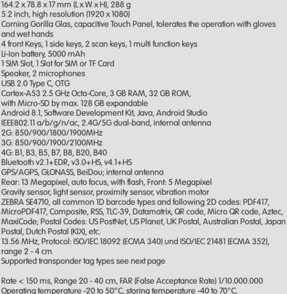
Operating temperature -20 to 50°C, storing temperature -40 to 70°C, relative humidity 5 to 95%, not condensing Multiple 1.8 m drops to the concrete across the entire temperature range and 1000 0.5 m drops at room temperature IP67
