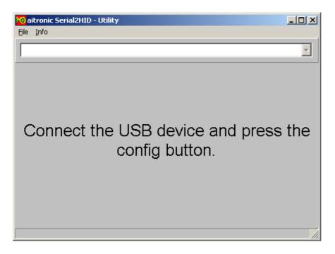
For configuration the Seriell HID Adapter has to be connected to a USB port. As soon as the Seriell HID Adapter's LED flashes green the reset button (5), behind the small hole beside the USB cable connection, has to be pushed one time (i.e. be means of a bended up paper-clip). After taht the LED flashes alternately green and red.
