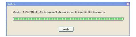
A progress bar will show the update process. At the end of the update the buttons text will change from "please wait" to "ready". The programmierung is completed and the ACR-320 will change to "capturing mode". All configuration settings are preserved after firmware update.
